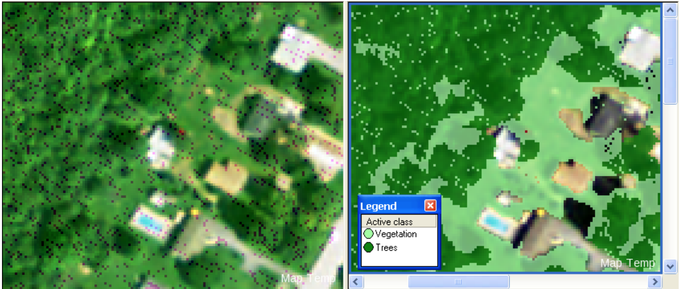
Figure 37: Optical layers and Number of Returns not interpolated in mixed view (left); classification results based on not interpolated data (right).
