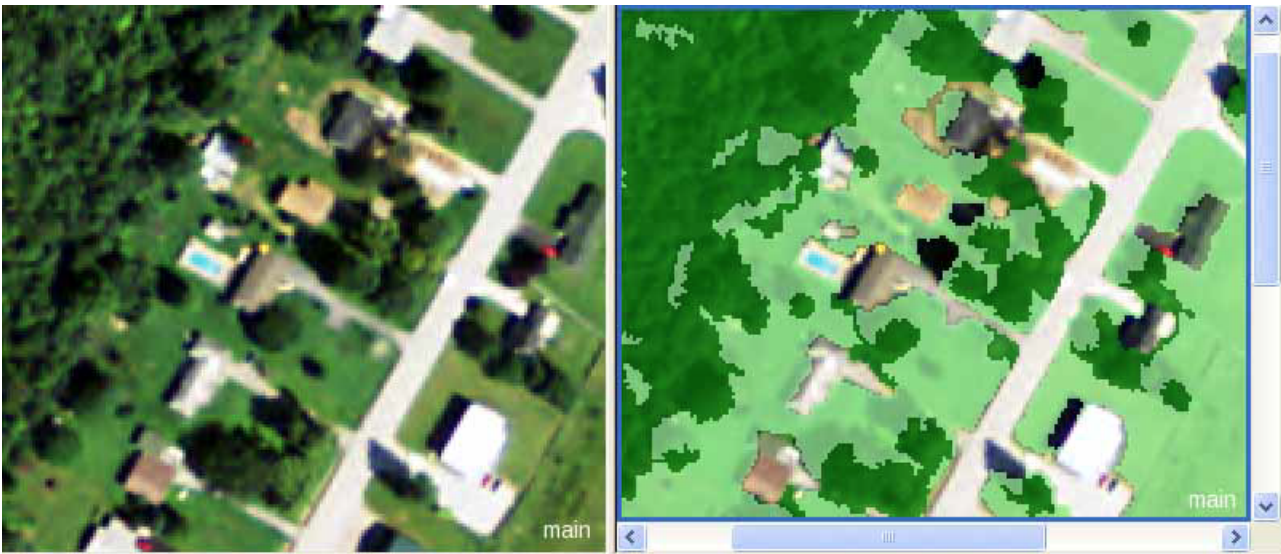
Figure 36: Optical layers (left); classification results using interpolated image layer 'Number of Returns Interpolated' (right).
