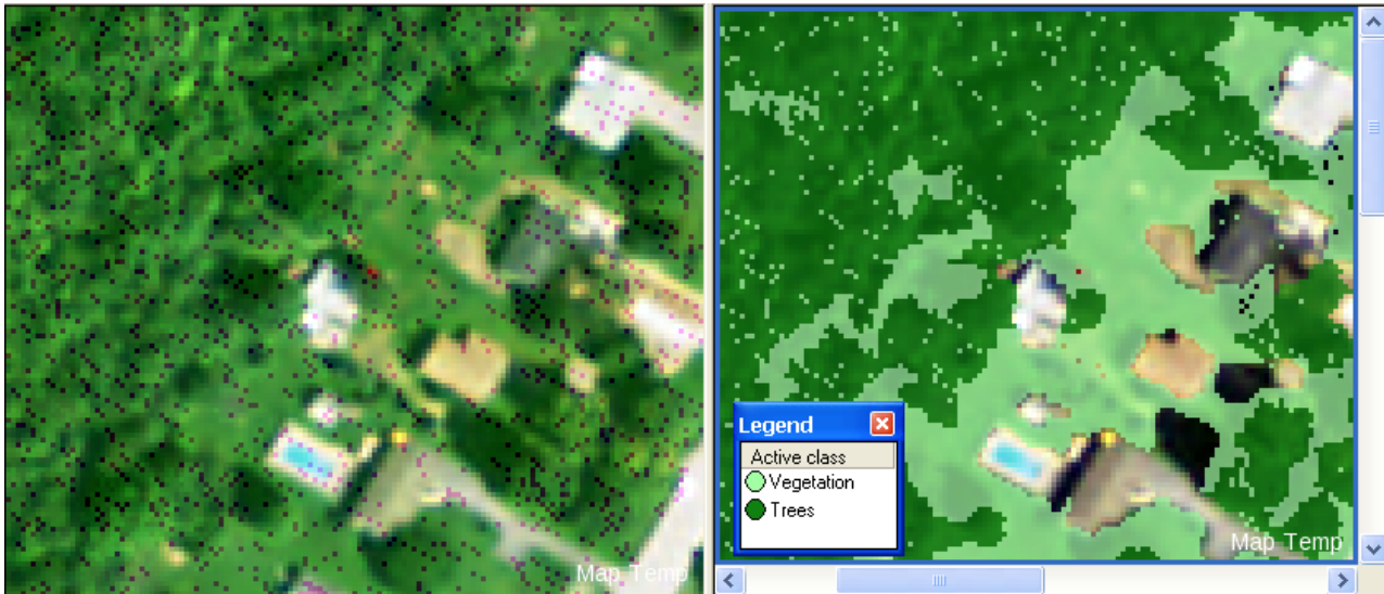
Figure 18: Optical layers and Number of Returns in mixed view (left); classification Result (right).
